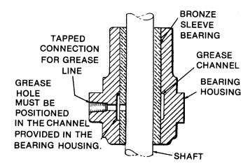
Figure 8. Installation of Sleeve Bearing for Types LB3A, LB3A, LB4A and LH2A
