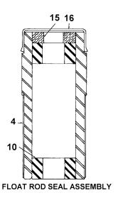
Figure 3. Float Rod Installation
