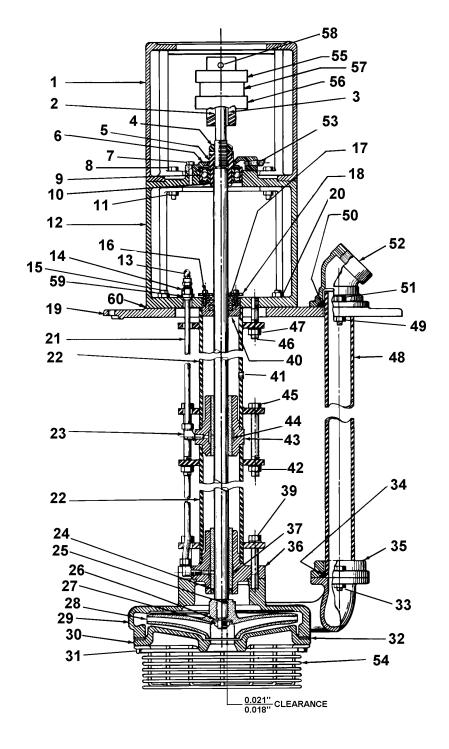
Figure 6. LH2A, LB3A, and LB4A Sump Pump
