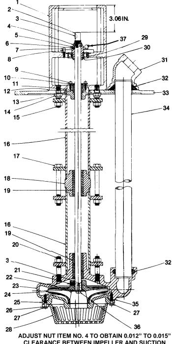
**CLEARANCE BETWEEN IMPELLER AND SUCTION CASING**
