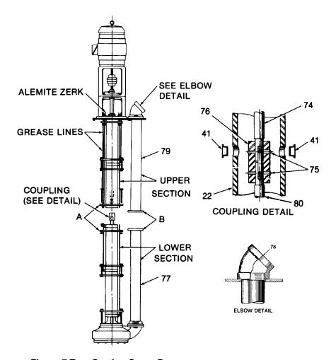
Figure 7 Two-Section Sump Pump
