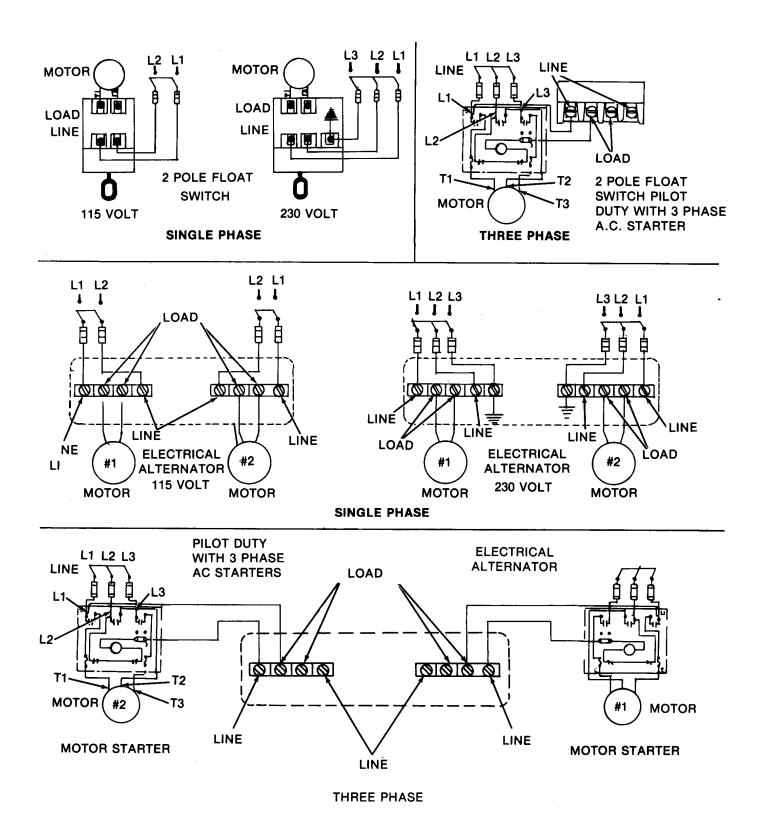
**Figure 4. Typical Control Wiring Diagrams**
