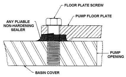
Figure 2 Sealing the Pump Floor Plate
