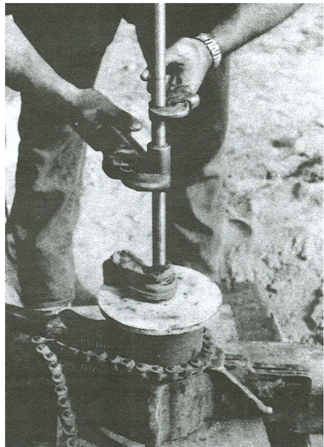
Fig. 7-7. Making A Shaft Joint. Special Protective Apron Placed Over Bowl Unit, With Clean Rag Wrapped Tightly Around Impeller Shaft.
